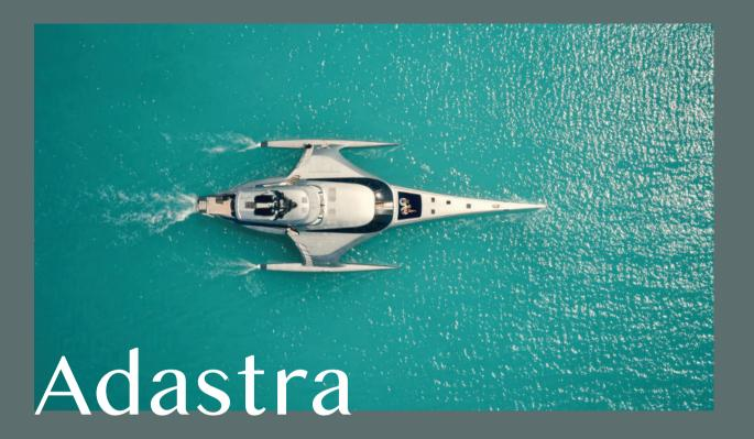
A cutting-edge trimaran, Adastra meaning "to the stars" in Latin, was specially designed for efficiency, stability and performance. Conceptualised in 2012 by leading race yacht builders, McConaghy Yachts, for island adventuring, a shallow draft of 1.2m (3.9ft) means the vessel can explore a wider range of harbours and islands, perfect for the turquoise shallow waters of the Maldives.
