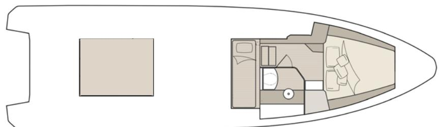
Length: 12,4 m / 40,7 ft, Beam: 3,55 m / 11,7 ft, Draft: 0,75 m / 2,5 ft, Passengers: B: 12, Max. engine power: 800 hp, Max. speed range: 35-45 knots, Fuel: 1000 L / 264 gal, Diesel for heater: 25 L / 6,6 gal, Fresh water: 210 L / 55 gal, Gray water tank: 105 L / 27,8 gal, Black water tank: 60 L / 15,8 gal, Construction: Vacuum infused GRP, Hull design: Twin-stepped V21° Hull
